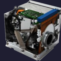
CUBECAT Laser communication terminal
